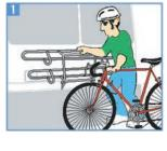
Pull down to release the folded bike rack. You only need one hand to pull the rack
